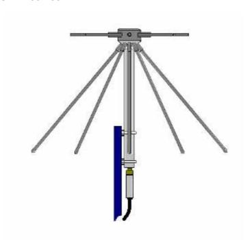
Designed for shipboard mounting, the BPV-SPB 100-400 is a compact vertically polarised broadband antenna which operates in the frequency range of 100-400 MHz with power handling of 300 watts CW. Antenna radiating elements are of marine grade stainless steel with a grey polyurethane lacquer finish. All other exposed surfaces are fully protected against aggressive, marine/ salt spray environments.
