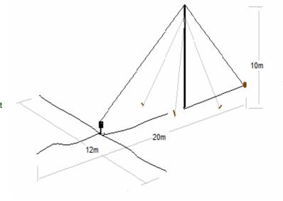
Supplied with kit is Model BPV-TM-35-8 **Tactical Mast**
